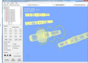
Among the main features of the Shaft Viewer is its ability to display and animate the motions calculated by the various ARMD solvers. When the Shaft Viewer loads a ROTLAT or TORSION shaft system model, it automatically looks for supported solver output files. No user interaction is needed. These output sets are then presented to the user for display in the *Output Set Property* drop-down box on the viewer's main toolbar.
