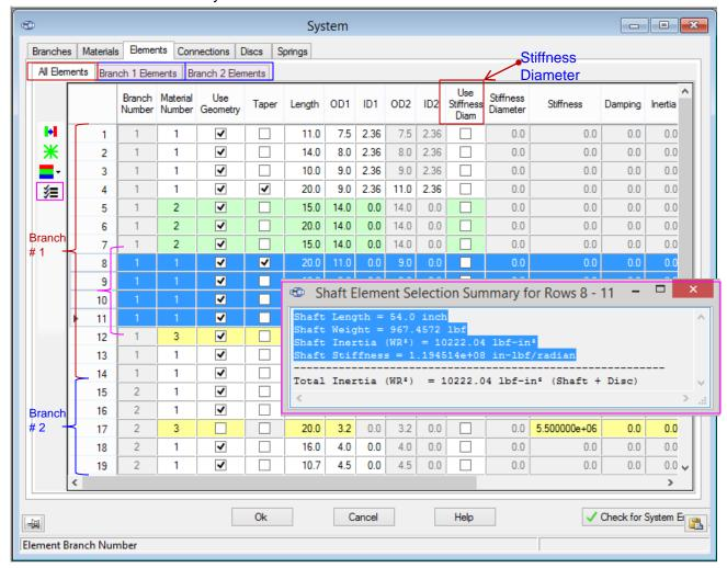
> Stiffness Diameter. Can be used to enter the equivalent mass-elastic properties of complex shaft sections, motor lamination stacks, shrunk on disks, etc.
