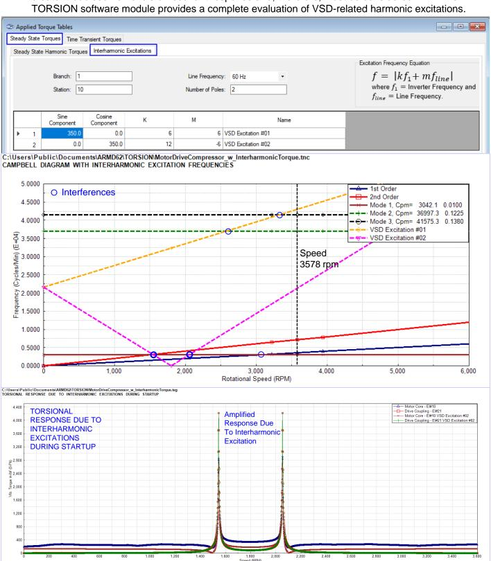
Generator/Motor Electrical Excitations. Among the features incorporated in TORSION package are electrically-induced, time-varying exciting torques associated with generator and induction motor operation that include:
