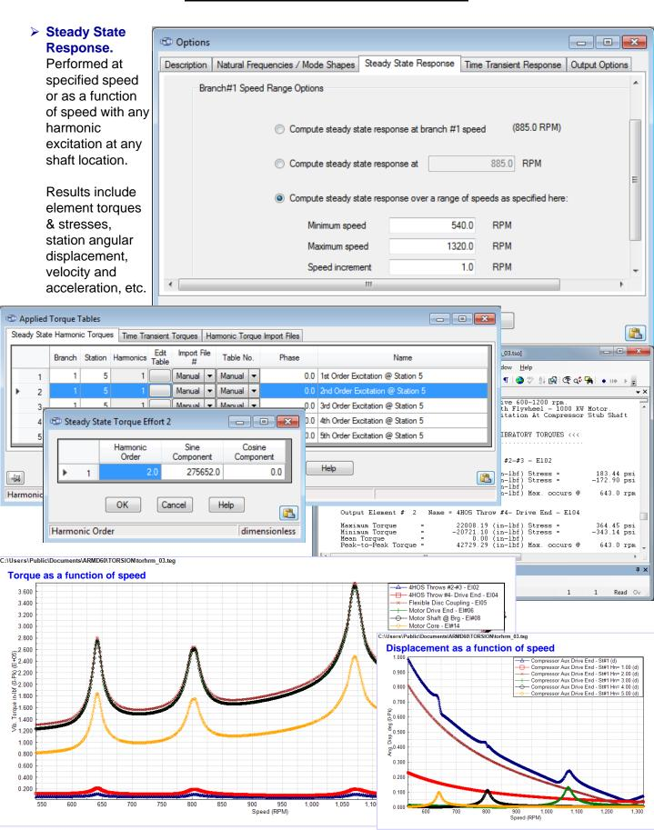
Steady State Interharmonic Excitation & Response. Electric motor controllers used in variable-speed drive (VSD) applications generate integer and non-integer harmonic torsional excitations. Intersections between these harmonic excitations with relevant torsional natural frequencies can create "troublesome" levels of resonant response and, therefore, must be considered. ARMD's TORSION software module provides a complete evaluation of VSD-related harmonic excitations.
