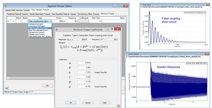
> Startup characteristics of synchronous motor, user-specified time-transient external-torques, & calculated system response torques are available in the graphics output file.
