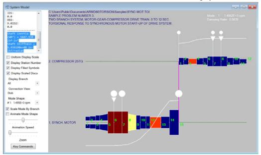
**2-D Model auto resizing** gives user the option to "fit-to-page" complete models or single branches. User can automatically view the model with the correct aspect ratio, thereby permitting rapid, visual model review.
