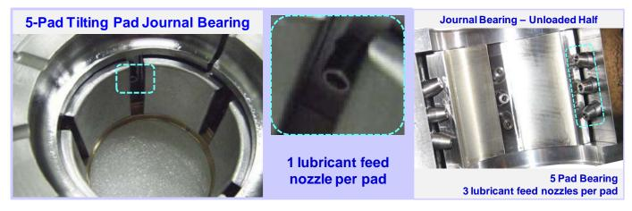
For "Pressurized" flow type, the supply pressure, number of orifices/nozzles per pad and orifice/nozzle geometry are specified by the user.
