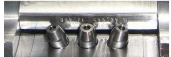
Illustration of Three Feed Orifices/Nozzles per Pad
