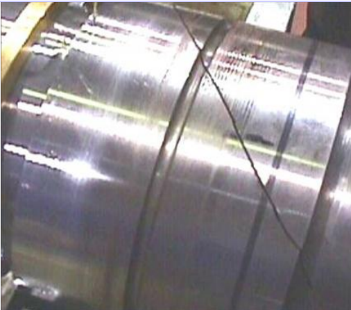
FORENSIC INVESTIGATIONS Torsional Failure in Motor Drive End Shaft
