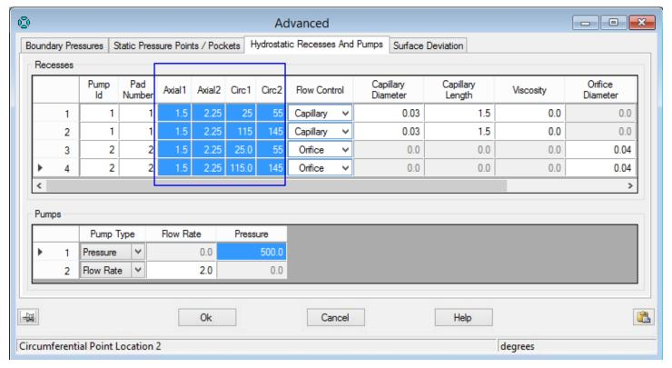
Hybrid bearing performance results are computed with each recess considered as having its own feeding system. The solution is bearing performance takes into account both the hydrostatic and hydrodynamic lubrication regimes, iteratively solving for flow and pressure in each recess.
