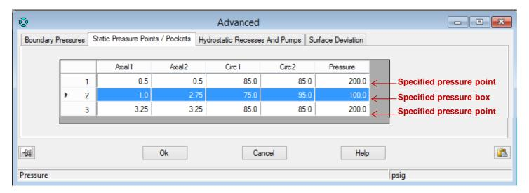
The above specified conditions illustrate (shown pictorially below with the display of the pad grid layout) the specification of point pressure at an axial location of 0.50 inches and located at 85 degree circumferentially, point pressure at an axial location of 3.25 inches and located at 85 degree circumferentially, as well as pressurized pocket/box bounded axially at 1.00 and 2.5 inches, and circumferentially at 75.0 and 95.0 degree
