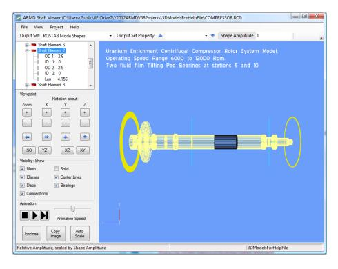
The main feature of the Shaft Viewer is its ability to display and animate the motions calculated by the various ARMD solvers. When the Shaft Viewer loads a ROTLAT or TORSION shaft system model, it looks for supported solver output files, and if they are present will load any or all of them automatically, no user interaction is needed. These output sets are then presented to the user for display in the Output Set: drop-down box on the viewer's main toolbar (shown below).
