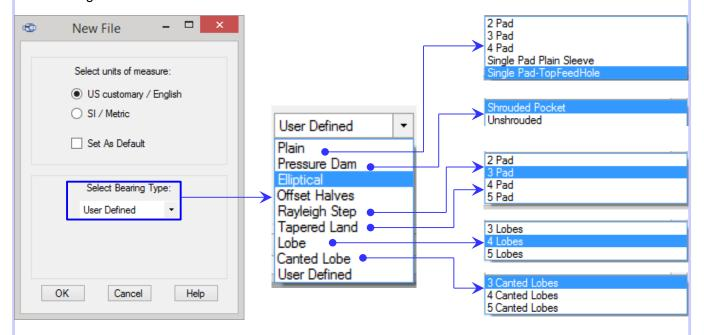
**Bearing Pad Configuration**. A vastly improved pad configuration tab allows the user to select from many standard bearing types, including special options, while restricting input to only those fields/cells pertinent to that type.
