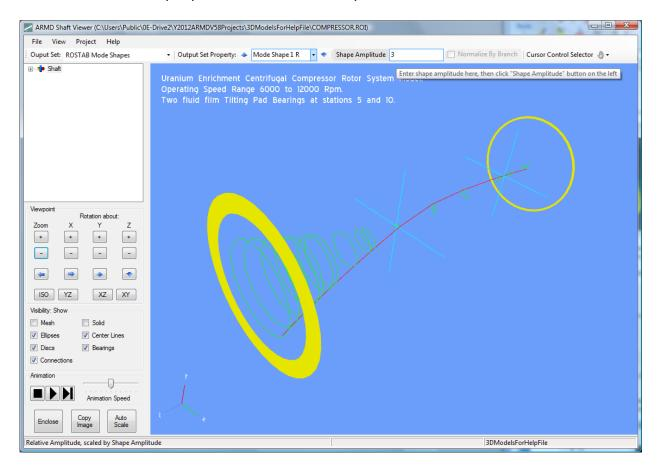
The red line represents the location of the center of the shaft at each station in the model. Animating this view can show better detail of the precise motions including relative phases at each station. This is accomplished by using the Visibility check boxes positioned right above the animation controls (also shown below).
