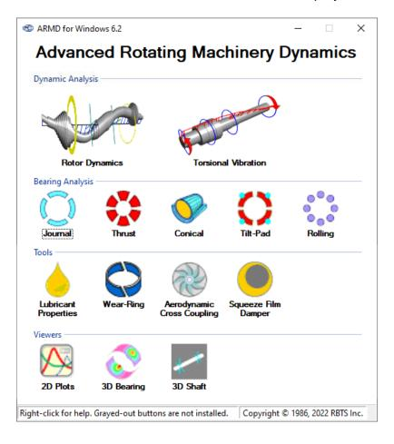
At this point, you are at the top level/menu of the software package. From this main menu, you can activate any of the preprocessor modules for bearings, bearing systems, rotor dynamics, torsional vibration, or lubricant properties calculation.
