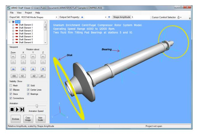
The Shaft Viewer can be run as a stand-alone display utility either from the ARMD main menu or from the computer's Start menu. It is also fully integrated into the ROTLAT Rotor Dynamics and TORSION Torsional Vibration modules, where it can be accessed via the View menu as shown below (if run from ROTLAT or TORSION, it will start with the model in use fully loaded).
