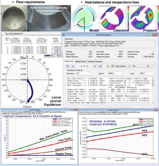
**Pre-Configured Bearing Types**. The newly developed package incorporates a significant number of preconfigured bearing types (templates) used in industry. When creating a new bearing model the built-in wizard and templates expedite the creation of bearing models and provide bearing performance results in few keystrokes. Users can create additional templates of their specific bearing configurations and utilize them during their normal work flow.
