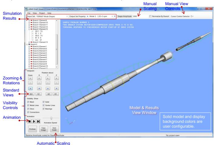
The Shaft Viewer can be run as a stand-alone display utility either from the ARMD main menu or from the computer's Start menu. It is also fully integrated into the ROTLAT Rotor Dynamics and TORSION Torsional Vibration modules, where it is automatically loaded/accessed via the View menu.
