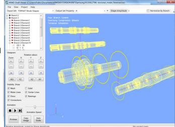
Among the main features of the Shaft Viewer is its ability to display and animate the motions calculated by the various ARMD solvers. When the Shaft Viewer loads a ROTLAT or TORSION shaft system model, it automatically looks for supported solver output files. No user interaction is needed. These output sets are then presented to the user for display in the *Output Set Property* drop-down box on the viewer's main toolbar.
