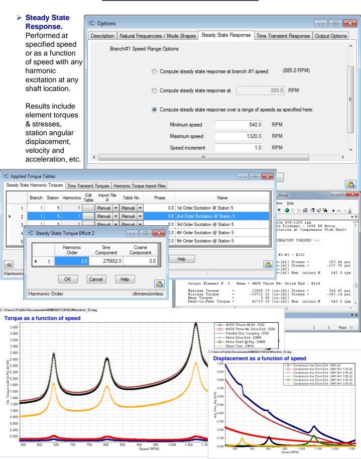
Generator/Motor Electrical Excitations. Among the features incorporated in TORSION package are electrically-induced, time-varying exciting torques associated with generator and induction
