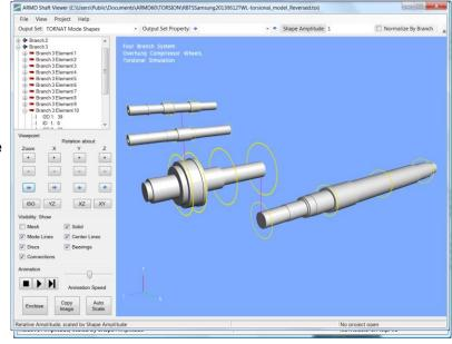
Various elements of the model can be selected for display using the check boxes in the Visibility control group. When Solid and Mesh items are selected, the viewer performs an automatic level-of-detail (LOD) calculation to determine when the mesh is too dense. If required, the software then suppresses the mesh display automatically.
