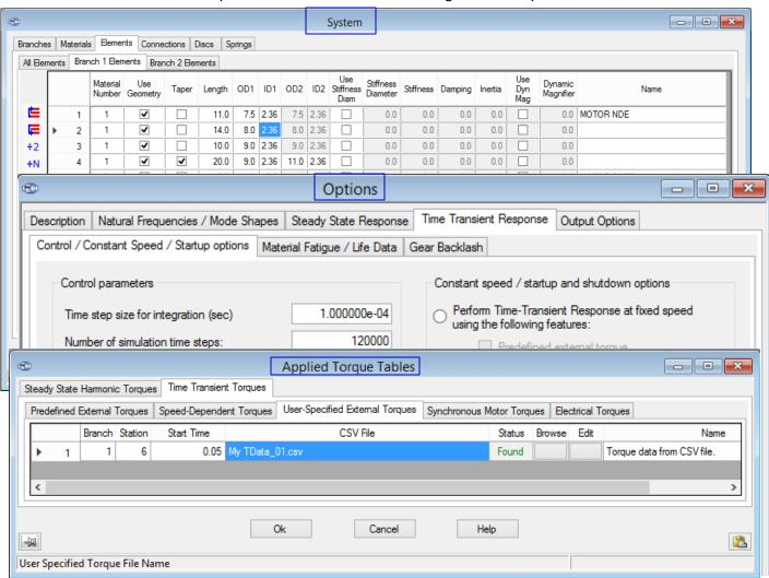
▶ Multiple instances of TORSION. The newly developed package can now open simultaneously multiple instances of TORSION, so shafts and component models can be moved easily between different models, also allowing fast, side-by-side comparison of model variations and analysis results. This functionality permits multiple instances of TORSION Version 6.0 or Version 5.8 to be accessible on your screens.
