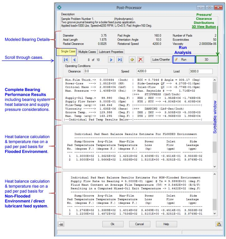
Multiple Cases / Parametric Evaluation: Multiple case bearing performance evaluation can be performed as a function of any combination of user defined operating conditions of Clearance, Speed, Load, Viscosity, Flow Rate, Temperatures, Pressure, Chamfers geometry, etc.
