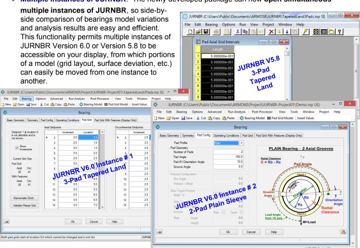
➤ User Configurable Expanded Toolbar. The main toolbar contains controls used to access frequently used functions (these functions are usually accessible from a menu as well). When a function is not available, its control on the toolbar will be disabled and displayed in a faded gray color. A user configurable expanded Toolbar has been added (second row of the toolbar shown below) for quick access to all of the View menu functions.
