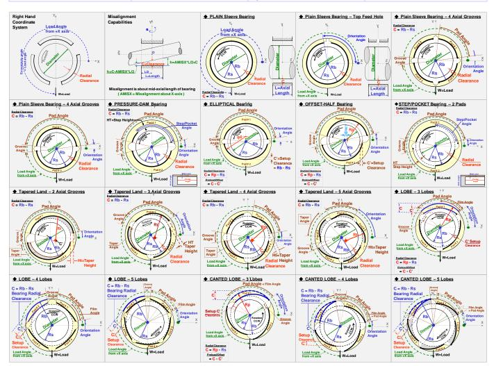
Simulation capabilities with **JURNBR** include such effects as misalignment, pressurized boundaries or grooves, cavitation, structural deformation/surface deviation, lubricant feed circuitry with specified pressures or restrictors (capillary, orifice, or flow control valve), groove geometry and chamfers to mention a few. Performance results include the following.
