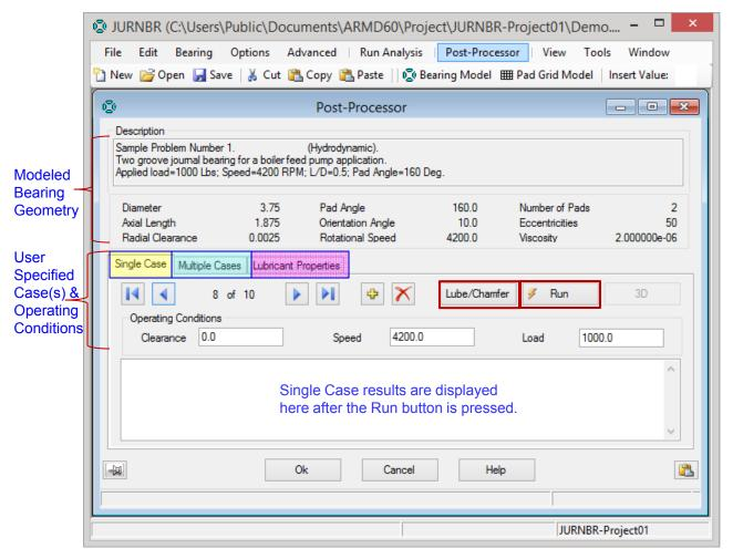
**Lubricant Properties** can be selected from the built-in lubricant data base or specified by the user. User specific lubricants, not available in the database, can be added for later retrieval / use.
